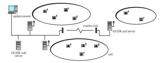
Figure 2.3: Lancaster GUIDE distributed architecture (Source: (Davies et al., 1999))
