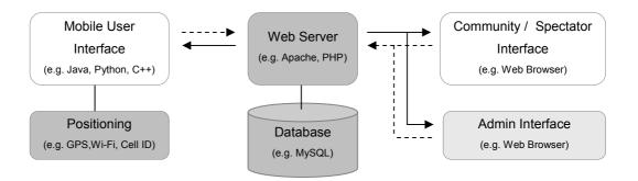
Figure A2.1: Example architecture of a custom mobile location-based game using standard components (Source: (Paelke et al., 2007))
