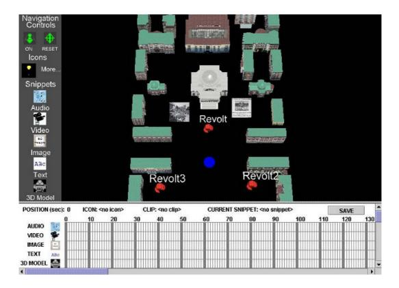
Figure 2.31: MARS Authoring Tool with 3D model of Columbia Campus, three defined locations (red), current user position (blue) and two image snippets (squares) (Source: (Güven and Feiner, 2003))
