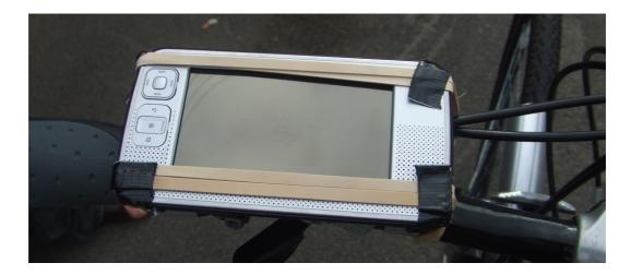
Figure 5.11: N800 mounted to bike with elastic straps and tape
