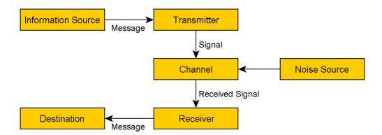
Figure A1.1: A general communication system according to Shannon
