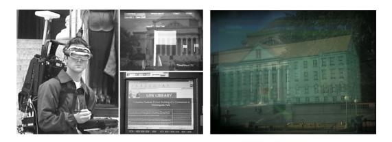
Figure 2.2: User with full kit (left), augmented view (top middle and right), browser view (bottom middle) (Source: (Höllerer et al., 1999))
