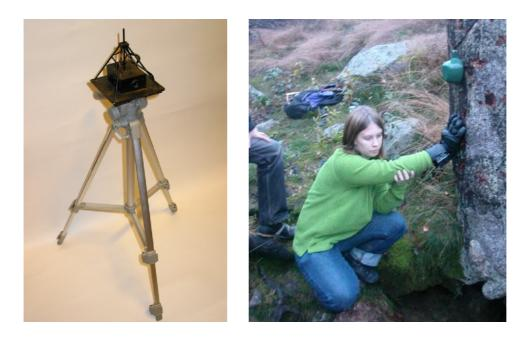
Figure 2.25: The Steele device with built-in Bluetooth GPS (left), the Thumin glove with built-in Bluetooth RFID reader in use by a player (right) (Source: (Hansson et al., 2007))
